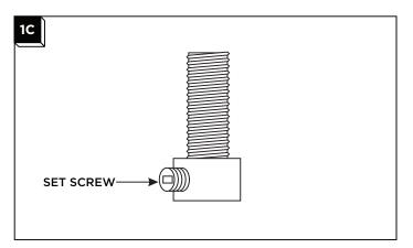
3 Loosen (Do Not Remove) the set screw on the strain relief.
