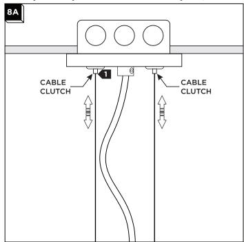
1 Adjust the aircraft cables until the fixture is level; feed the cable into the cable clutch to raise the fixture and push in on the cable clutch nipple to release the cable and lower the fixture.
