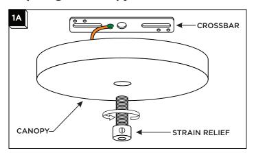
Remove the crossbar from the canopy by completely unscrewing the strain relief.
