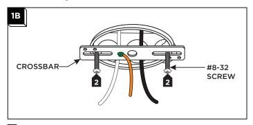
2 Mount the crossbar assembly to the electrical box with the two provided #8-32 screws.
