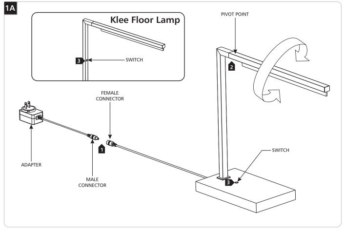
1 Connect the male connector from the adapter to the female adapter on the fixture.
