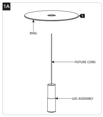
1 Feed the fixture cord through the ring and carefully lower the ring onto the LED assembly.
