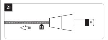
**12** Pull the coaxial cable toward the fixture to smooth the wrinkles.
