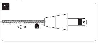
2 Pull the coaxial cable toward the fixture to smooth the wrinkles.
