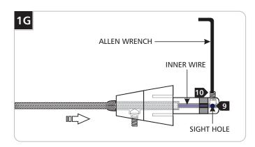
Look into the sight hole on the top of the connector to make sure that the inner wire is contacting the end of the connector.
