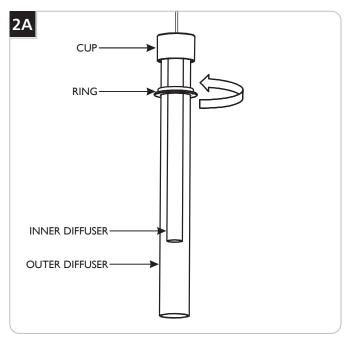
Insert the inner diffuser into the cup followed by the outer diffuser, then slide the ring over the outer diffuser and screw it into the cup to secure in place.
