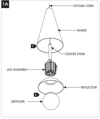
Feed the fixture cord through the shade then gently rest the inner shade on the center stem.
