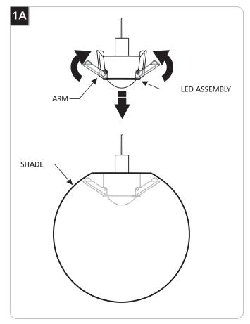
Fold and hold the arms, insert the LED assembly into the shade, center the LED assembly to the shade and release the arms. Adjust as necessary.
