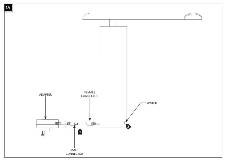
Connect the male connector from the adapter to the female adapter on the fixture.
