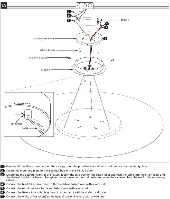
8 Connect the black driver wire(s) to the hot power line wire with a wire nut.
