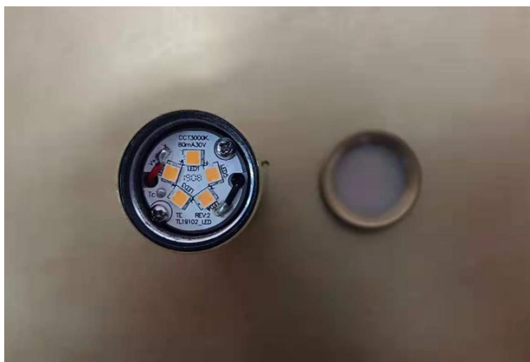
Internal view of 700LSPNT50*-LED930
