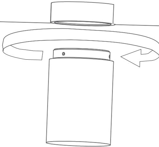
16 Install the shade by screwing into the shade base. Repeat for remaining shades.
