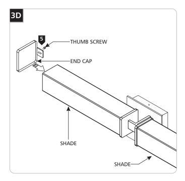
5 Reinstall the end caps to the ends of the shades and secure them using the two thumb screws.
