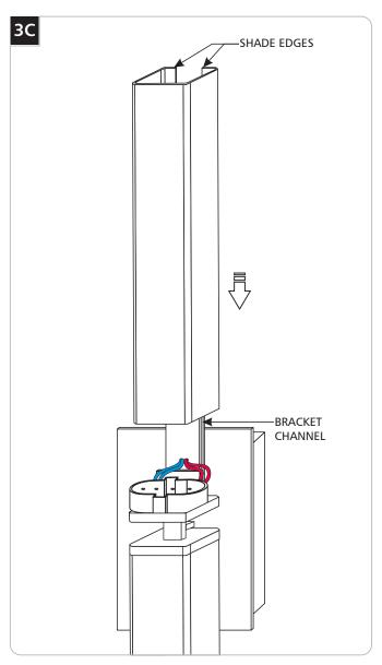
4 Carefully slide the shade edges into the bracket channels.
