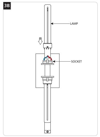
**CAUTION**: To reduce the risk of a burn or electric shock during relamping, disconnect the power to the fixture by turning the wall switch off.
