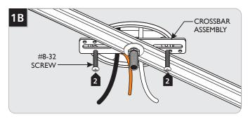
**Note:** If necessary, loosen the nut on the crossbar to adjust it to the desired position.
