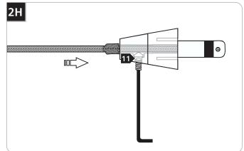
**1** Firmly tighten the set screw on the conical connector.
