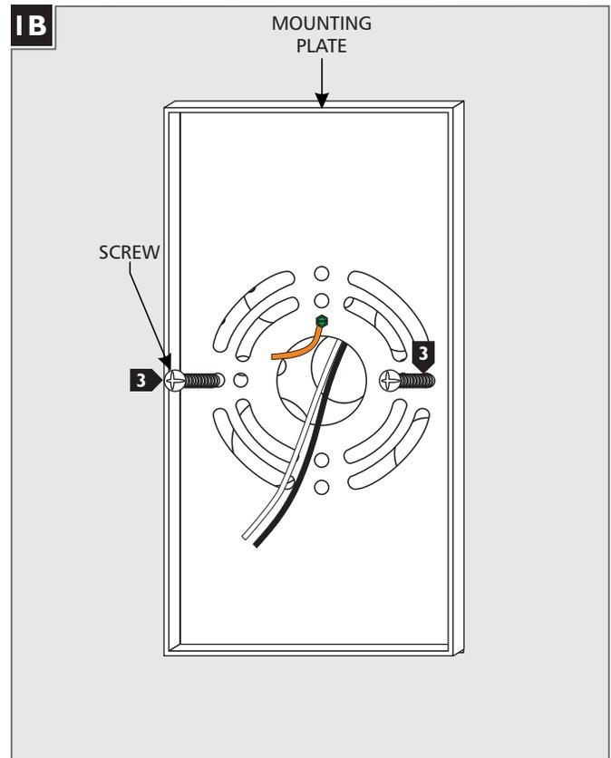
**3** Attach the mounting plate to the electrical box using the two #8-32 screws provided.
