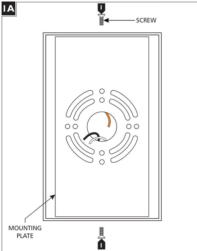
**1** Remove the two fixture screws on the top and bottom of the fixture.
