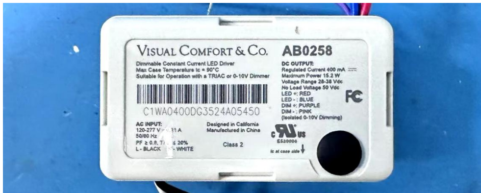
View of LED driver PTB20W-0400-38-VCC1(AB0258)
