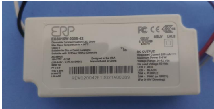
View of LED Driver ESS010W-0200-42
