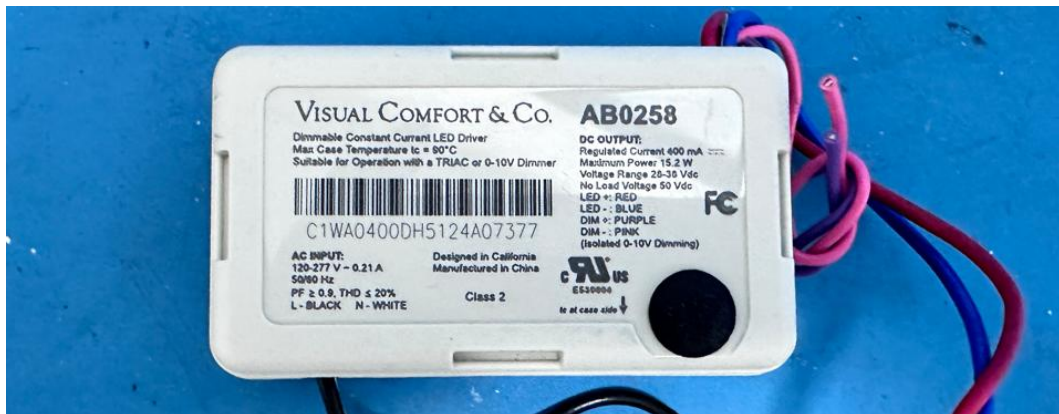
View of LED driver PTB20W-0400-38-VCC1(AB0258)
