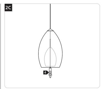
Use MAX 35 Watt Bi-Pin Halogen Lamp.
