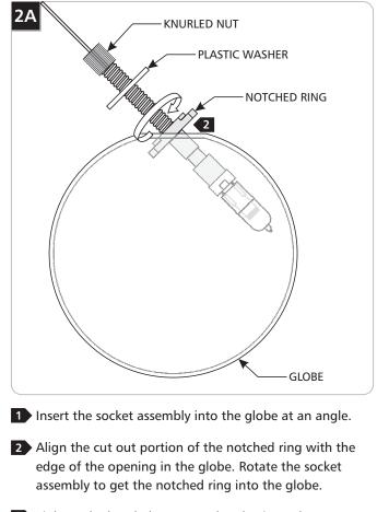
**3** Tighten the knurled nut onto the plastic washer.
