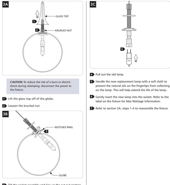
Tilt the socket assembly and line up the cut out portion of the notched ring with the edge of the opening in the globe. Rotate the socket assembly to get the notched ring out of the globe.
