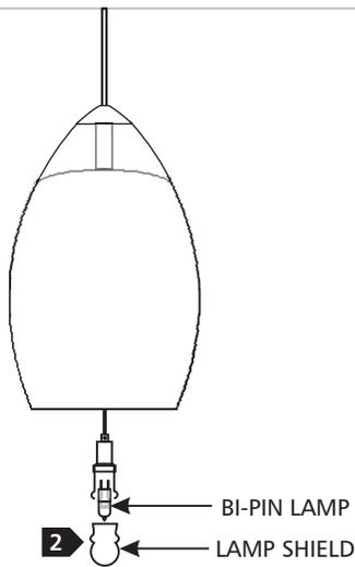
**2** Remove the lamp shield and the old lamp.
