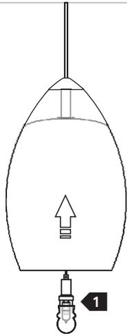
**1** Lift the glass shades up to expose the socket.
