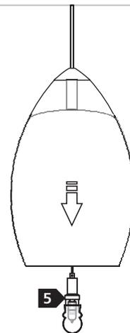
**5** Push the lamp shield onto the spring clip.
