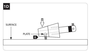
Tap the conical connector on a hard surface with the set screw facing down, so the plate inside drops into place.
