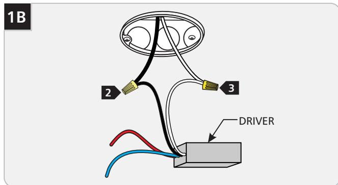
**2** Connect the black driver wire to the hot power line wire with a wire nut.
