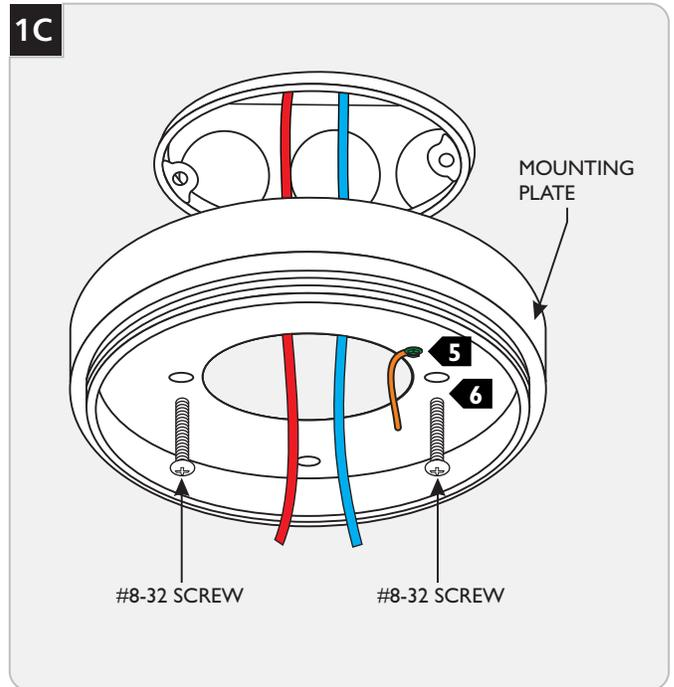
**4** Properly place the driver and wire connections into the electrical box.
