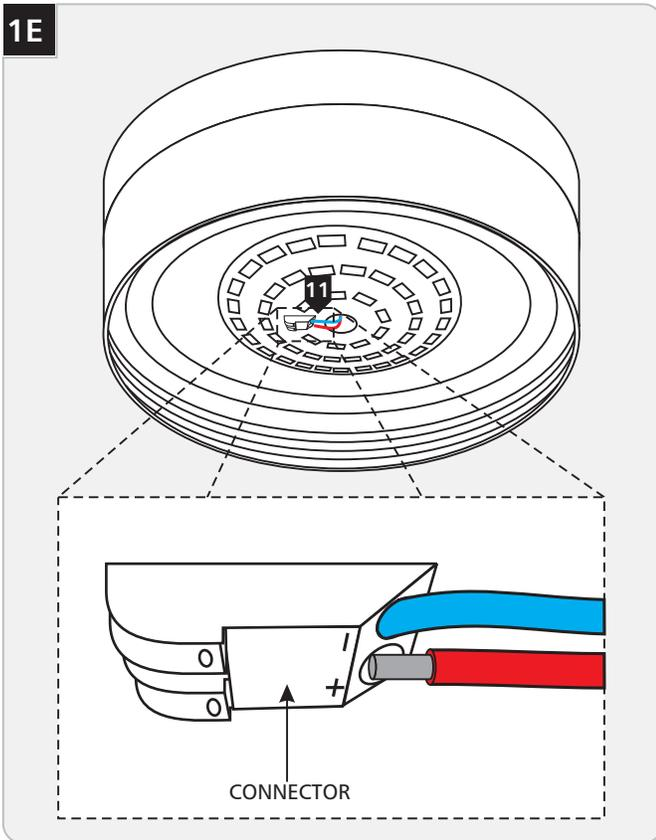
**8** Completely install the blue transformer wire to the negative terminal to make a connection.
