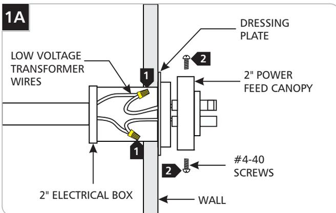
**NOTE:** 2" Electrical box should be installed prior to these steps. Refer to the instructions provided with the 2" electrical box.
