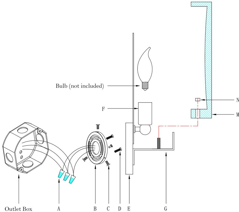
1. Remove mounting plate (B) from fixture base (E) by loosening the side screws (C).
