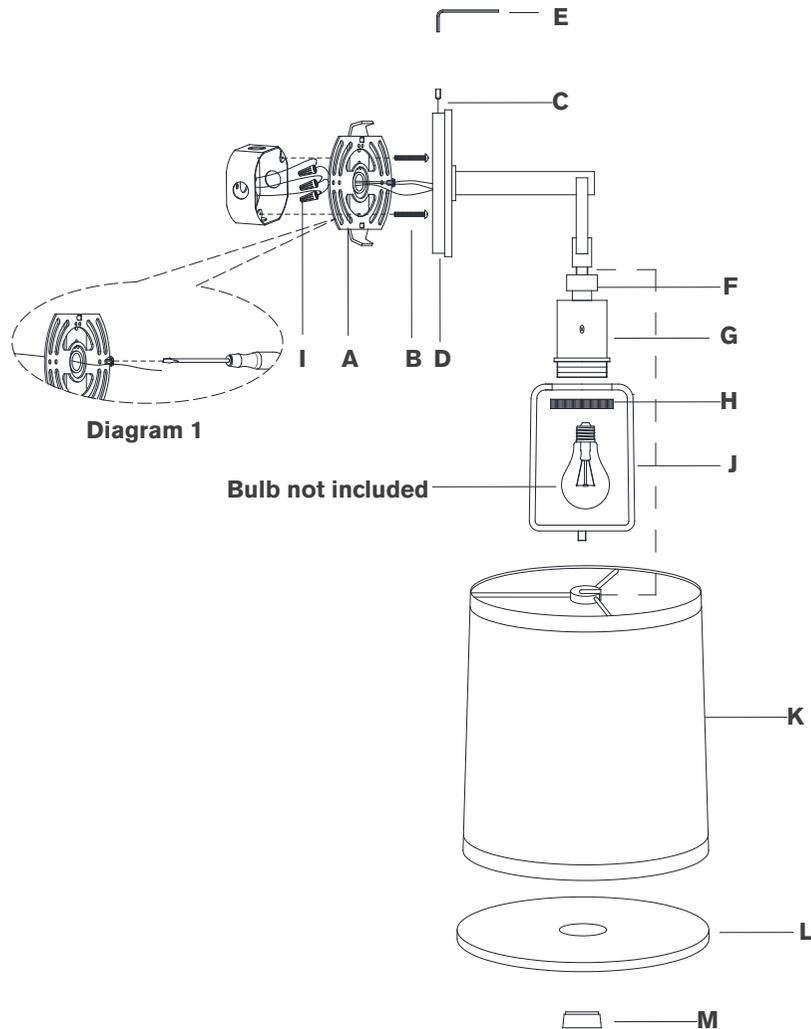
9. Install shade (**K**) to fixture body and secure with check ring (**F**).
