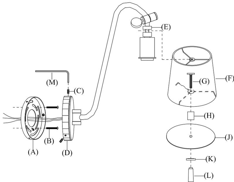
1. Remove diffuser (J) from lamp shade (F) by unscrewing washer (K) and finial (L).
