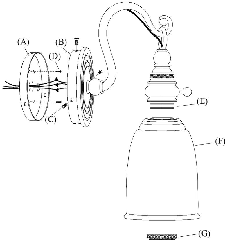
1. Remove back plate (A) from the base of lighting fixture (B) by unscrewing base screws (C) in counter-clockwise direction.
