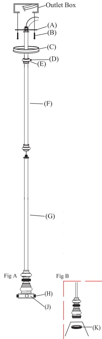
1. Loosen set screw (D), lower break (E) and canopy (C).
