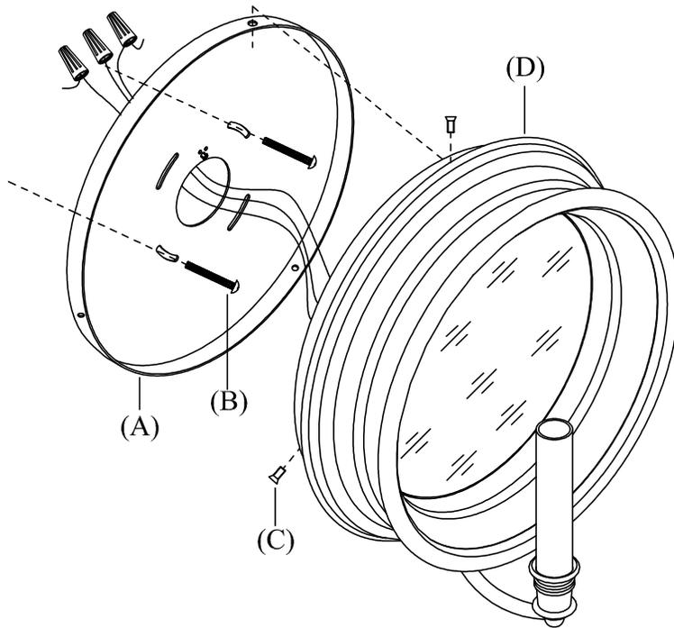
1. Attach the ground (green) wire to the ground wire from the wall outlet box (usually green or copper in color), and fasten together with a plastic wire connector. Tightly wrap the wire connector with electrical tape so the end of the connector is sealed. IT IS IMPERATIVE THAT THE OUTLET BOX IN YOUR HOME BE PROPERLY GROUNDED.
