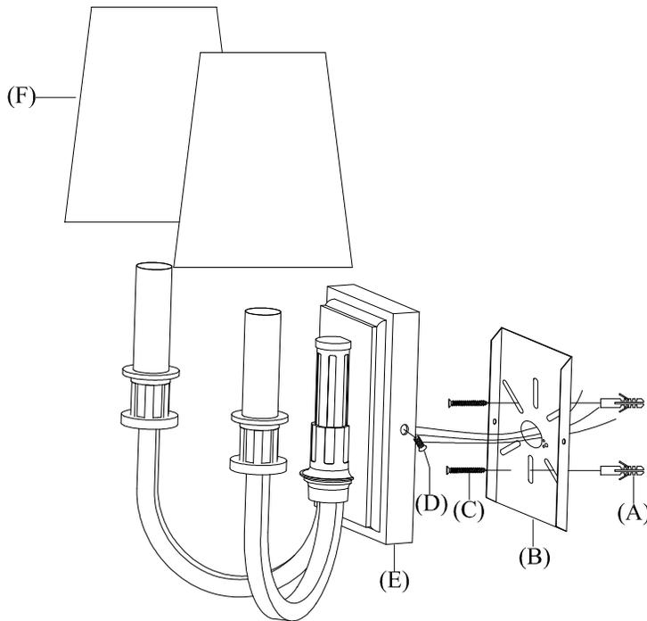
1. Remove back plate (B) from fixture base (E) by removing base screws (D).
