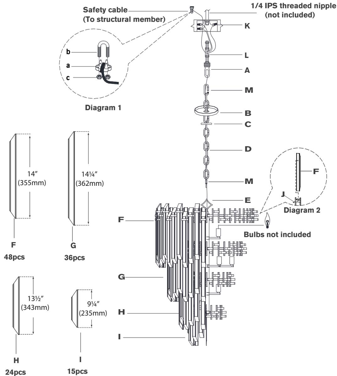
10. Twist all fixture wires together. Slip through center hole of collar loop **(A)**.
