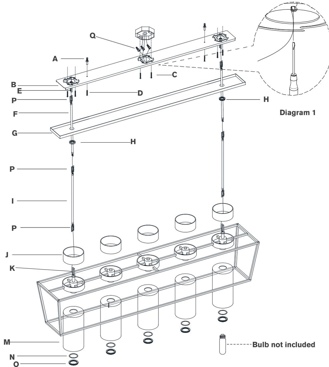
9. Connect bottom rods (**I**) to top rods (**F**), then attach to fixture loops (**K**) and hooks (**E**). Secure links (**P**) at ends of rods.
