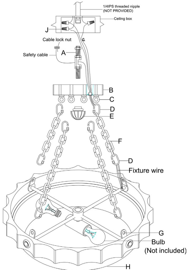
1. Install the threaded nipple (A) with hickey and nut into the top ceiling box. You must provide a 1/4 IPS threaded nipple which will go through the top of ceiling box and through a structural member of building.
