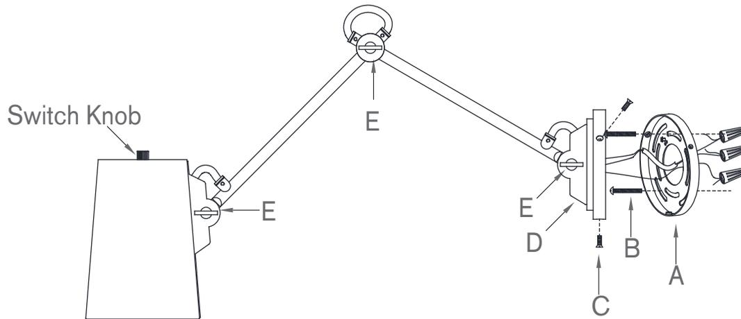
7. Attach fixture base (D) to the affixed mounting plate (A) and secure with base screws (C).
