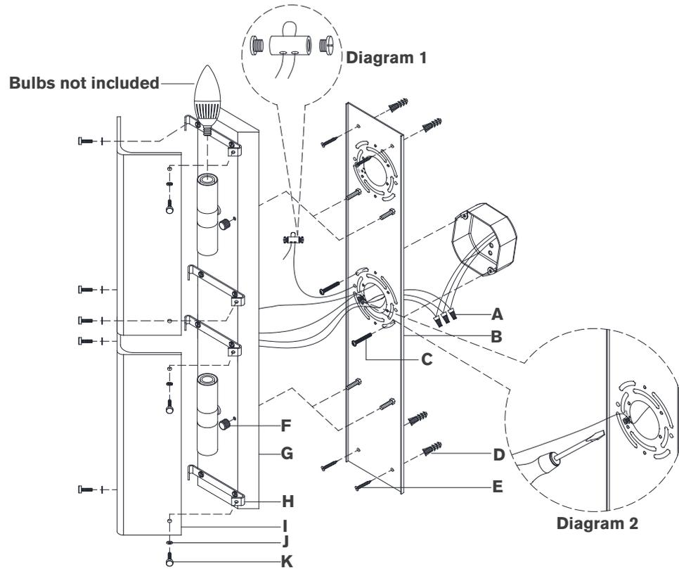
9. Connect fixture hot wire (black) to the supply hot wire (usually black) using wire nut **(A)**.
