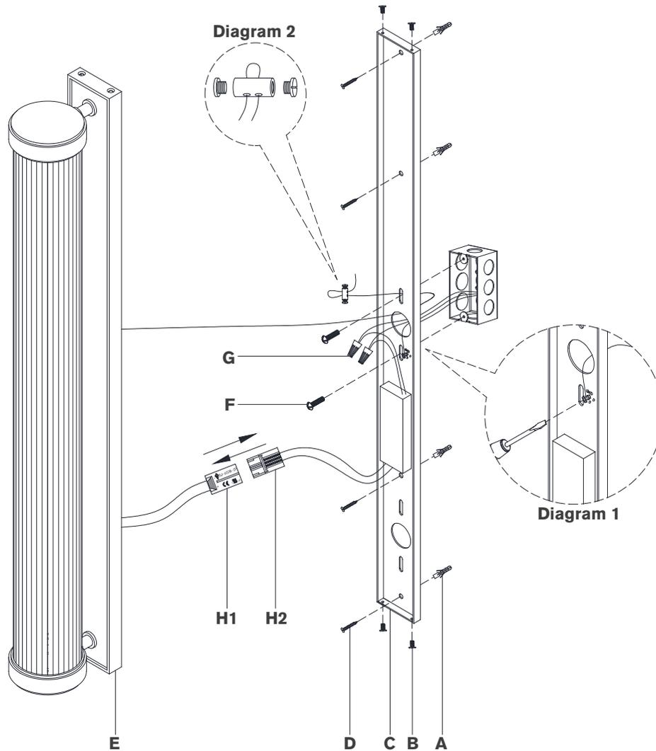
10. Make sure all wire connections are tight, then carefully tuck into the junction box.
