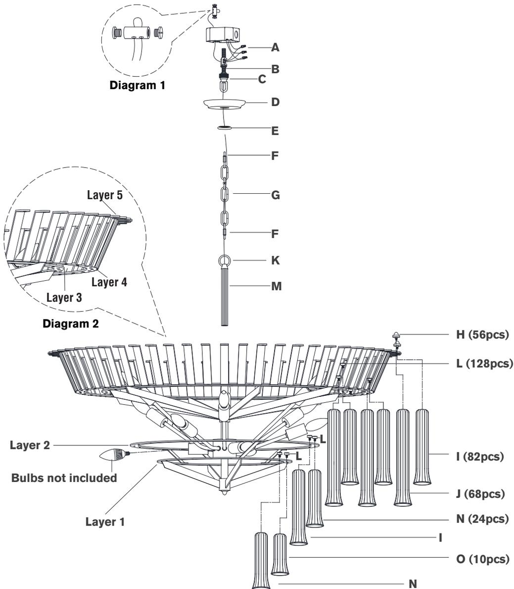
11. Twist all fixture wires together. Slip through center hole of collar loop (C).
