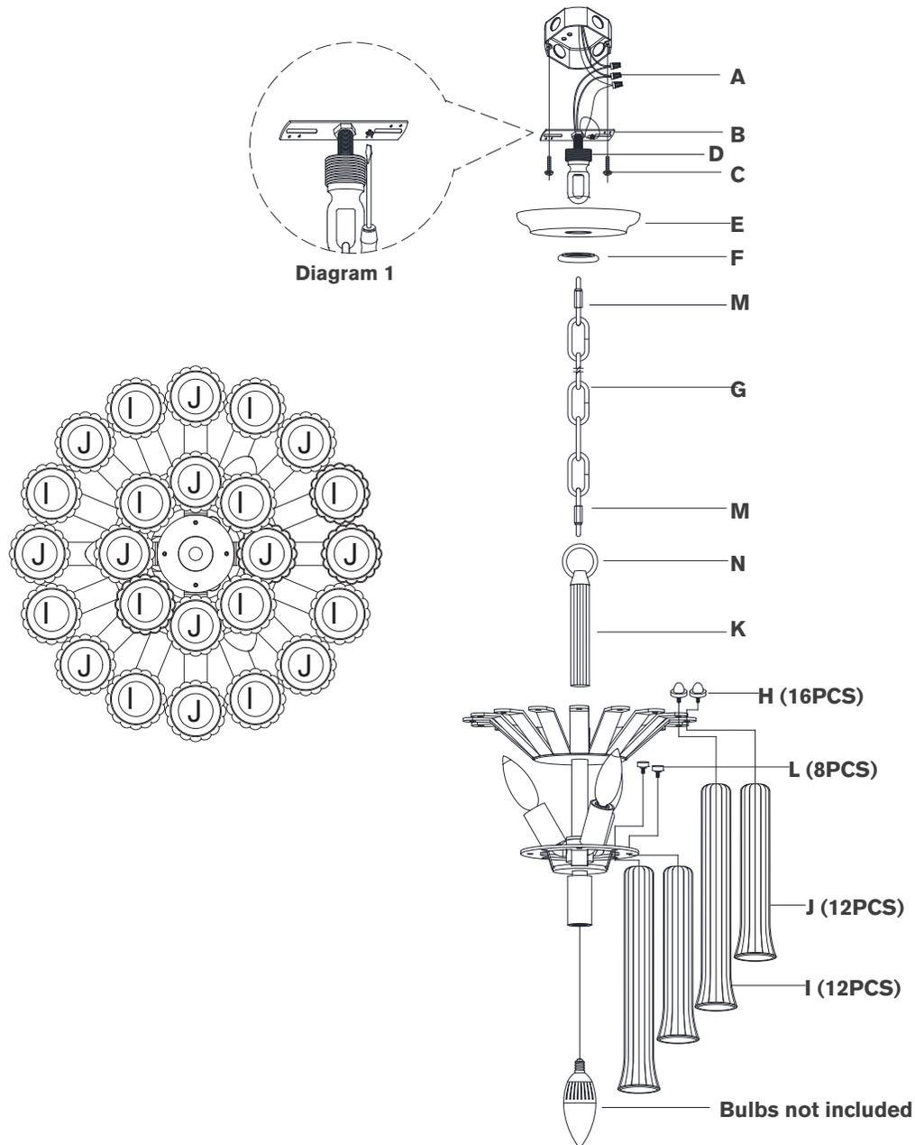
13. Wrap fixture ground wire (bare copper) around the green grounding screw (see diagram 1). Tighten. Continue fixture ground wire and connect to supply ground wire (usually green or bare copper) using wire nut **(A)**.
