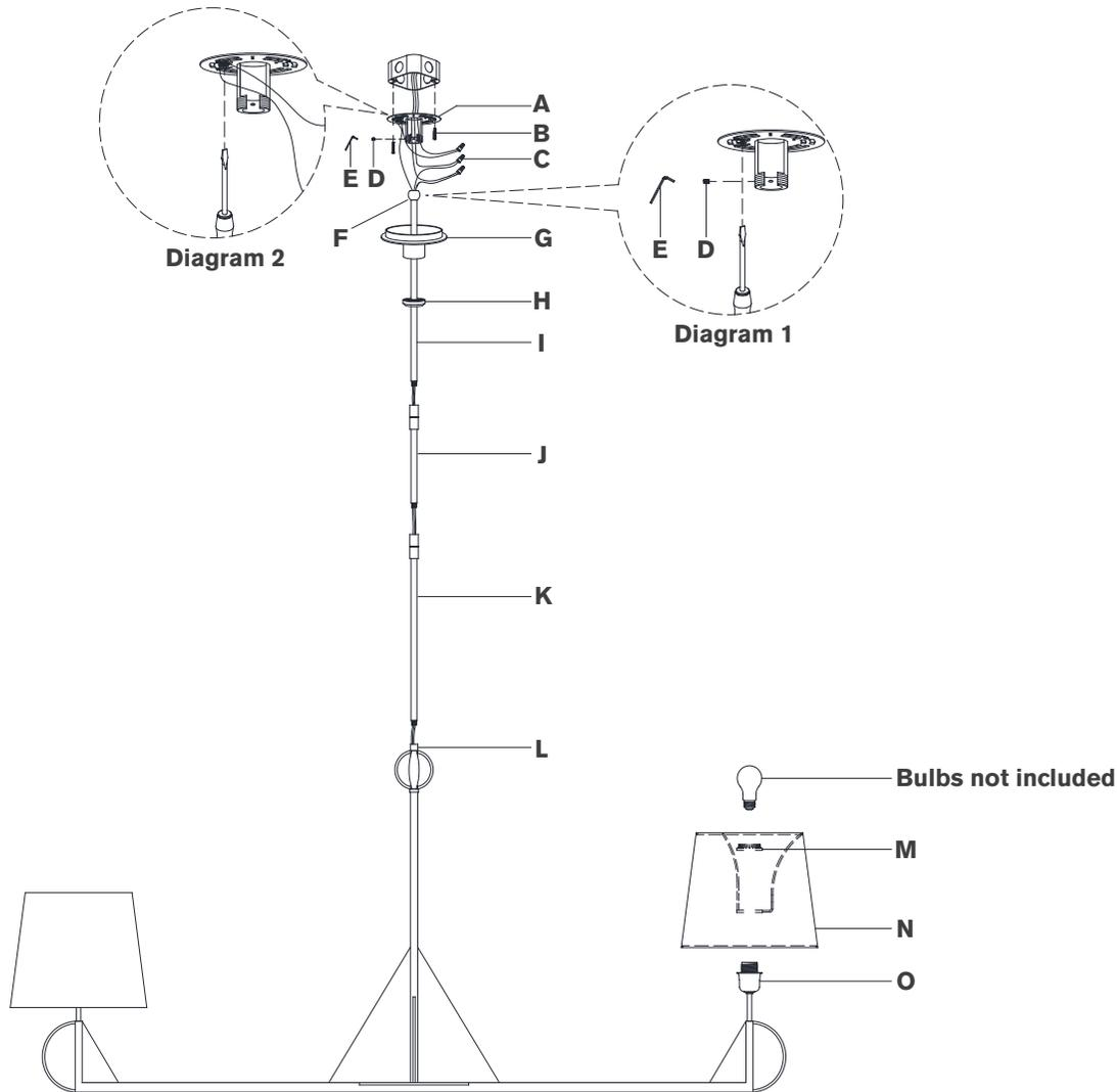
10. Connect fixture neutral wire (white) to the supply neutral wire (usually white) using wire nut **(C)**.
