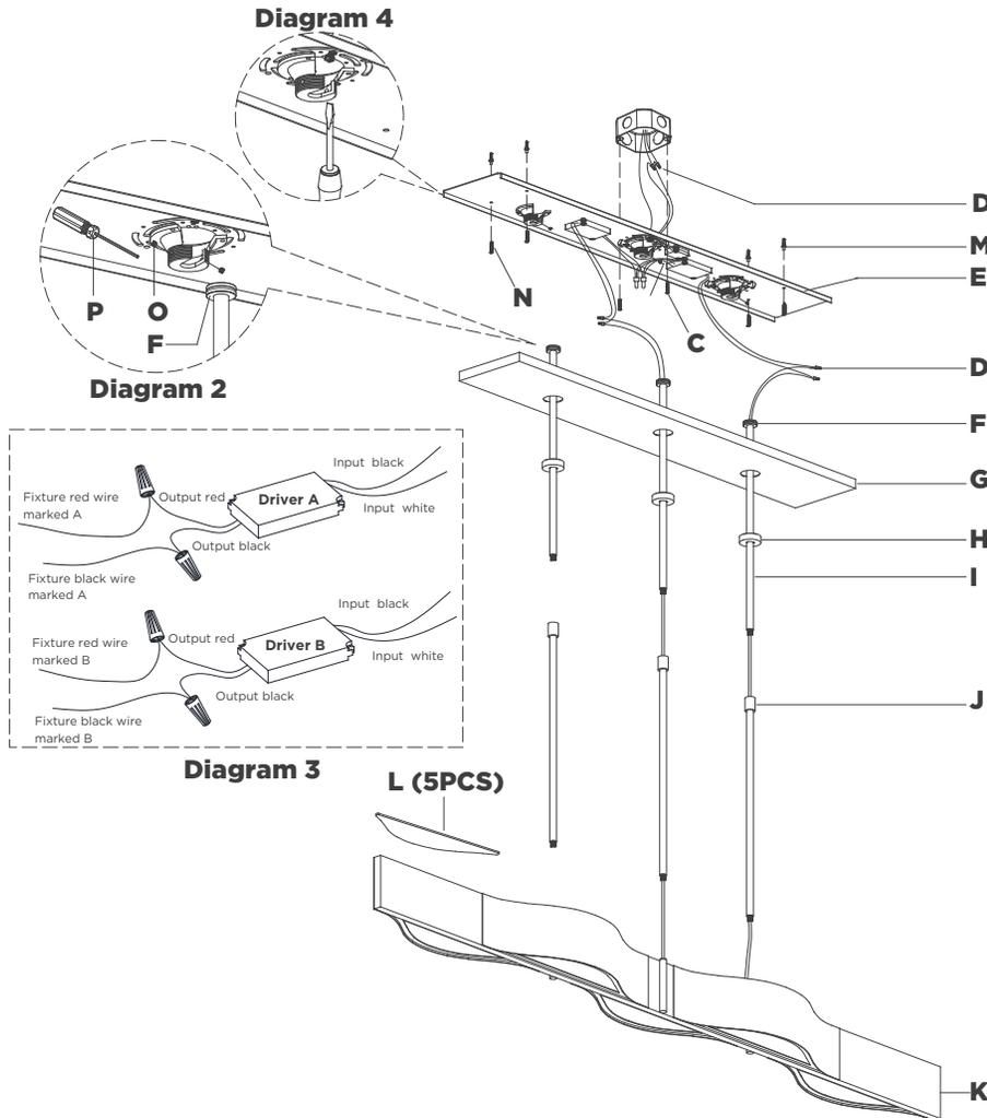
10. Hang fixture fan mounts **(F)** to center of mounting plate **(E)** and secure with set screws **(O)** using provided wrench **(P)** (see diagram 2).
