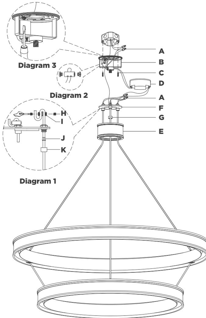
16. Connect driver **(D)** input hot wire (black) to the supply hot wire (usually black) using wire nut **(A)**.
