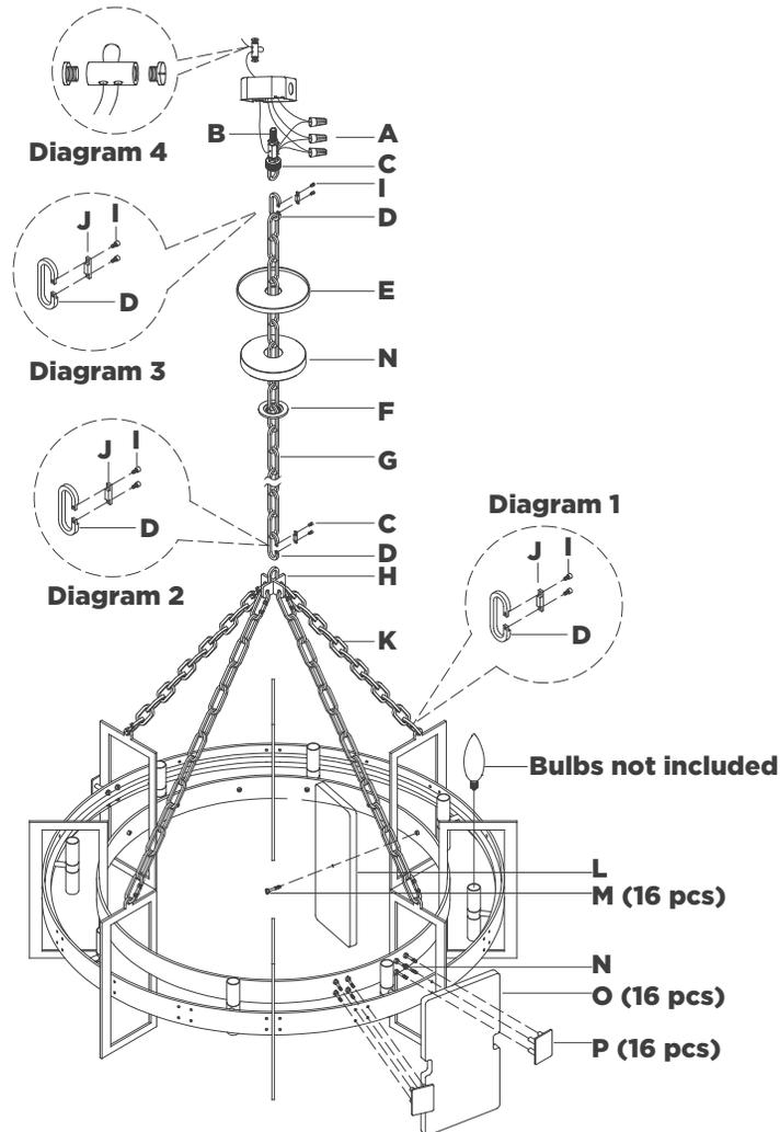
19. Install glass sheets **(L)** to inner fixture frame and secure by securing thumb screws **(M)**. Tighten thumb screws **(M)**.
