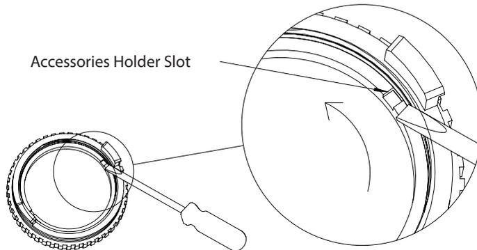
4. Fixture accommodates one lens and one glare control accessory. Refer to spec sheet for list of compatible accessories. Install accessories between the front cap and accessory holder. Tighten accessory holder after accessories are installed. **(Fig.7)**
