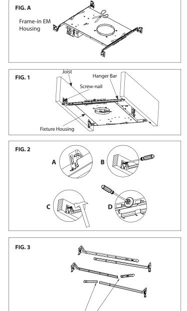
Snap off one section fit in a 12" joist
