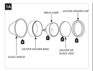
Use **MAX** 50 Watt MR16 Front Cover Halogen Lamp.
