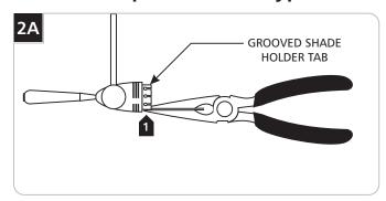
1 If the glass shield fits tight onto the fixture, then carefully bend the grooved shade holder tabs in slightly with the needlenose pliers. If it fits loose, then carefully bend the grooved shade holder tabs out slightly with the needlenose pliers.
