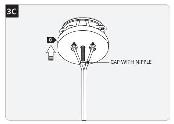
Slide the canopy up and secure it to the electrical box by screwing the cap with nipple to the crossbar.
