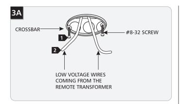
**NOTE:** Low voltage wires must be present in electrical box before proceeding with these steps. Refer to the instructions provided with the remote transformer.
