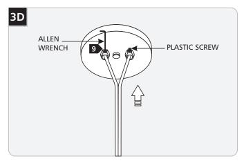
**9** Push the excess power feed wires into the canopy and tighten the plastic screw with the provided Allen wrench.
