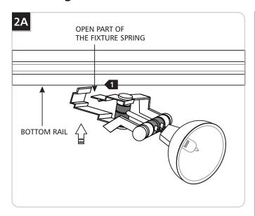
Push the open part of the fixture spring onto bottom rail.
