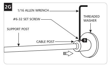
Push the support rod all the way into the support post and tighten the #6-32 set screw with the 1/16 Allen wrench.
