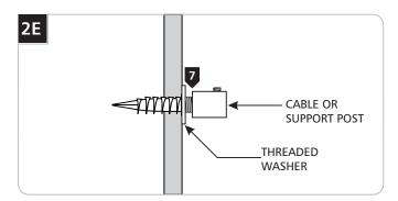
**7** Screw the cable and support posts to the threaded washers.
