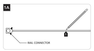
1 From the end without the rail connector, mark the section of the support rod that needs to be shortened.
