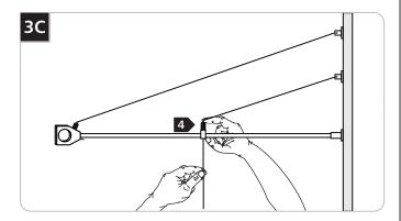
4 Support outside riggers with over 36" support rod come with an additional wire grip in the middle of the support rod. Repeat the applicable steps for installing the additional wire grip.
