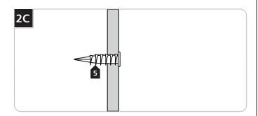
Screw the anchors in the rest of the way with a Phillips screwdriver.
