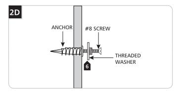
6 Attach the threaded washer to the anchor with the #8 screw.
