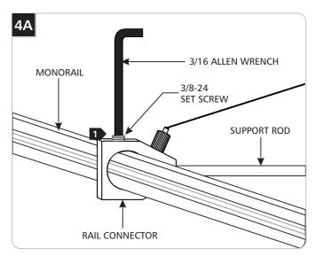
Slide the MonoRail through the rail connector hole and tighten the 3/8-24 set screw with the 3/16 Allen wrench.
