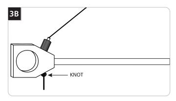
Put a knot in the aircraft cable beneath the rail connector when the angle is less than 30° or when the aircraft cable slips.
