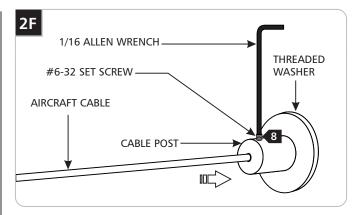
8 Feed the aircraft cable into the cable post and tighten the #6-32 set screw with the 1/16 Allen wrench.
